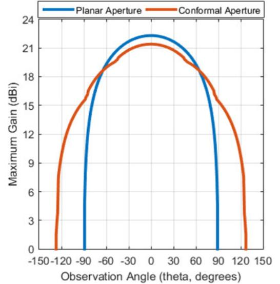
Fig. 6. Comparison of maximum theoretical gain against angle from broadside for conformal aperture, and planar array of the same area.
