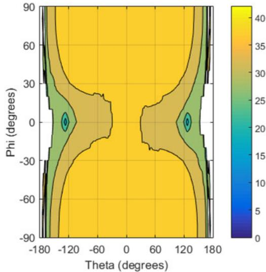
Fig. 8. Contour plot of the maximum gain pattern of the leading edge array, 5-dBi contours.
