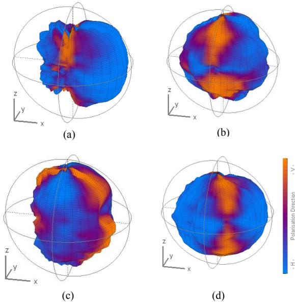
Fig. 3: Dipole Antenna on: (a) Chest, Top of wrist: (b) Hand forward, (c) Hand in front of chest, and (d) Side Arm-top.
