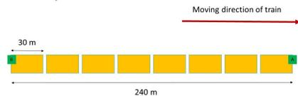
Fig. 2. Train considered traveling on the rail track
