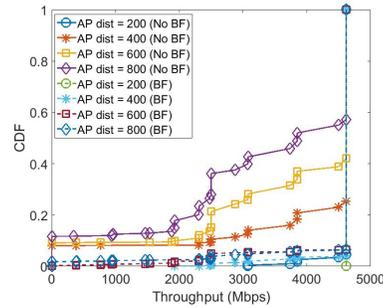
Fig. 7. CDF of Max. Throughput at 60GHz
