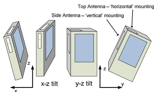
Fig. 1. Antenna element positions on terminal and elevation tilts.
