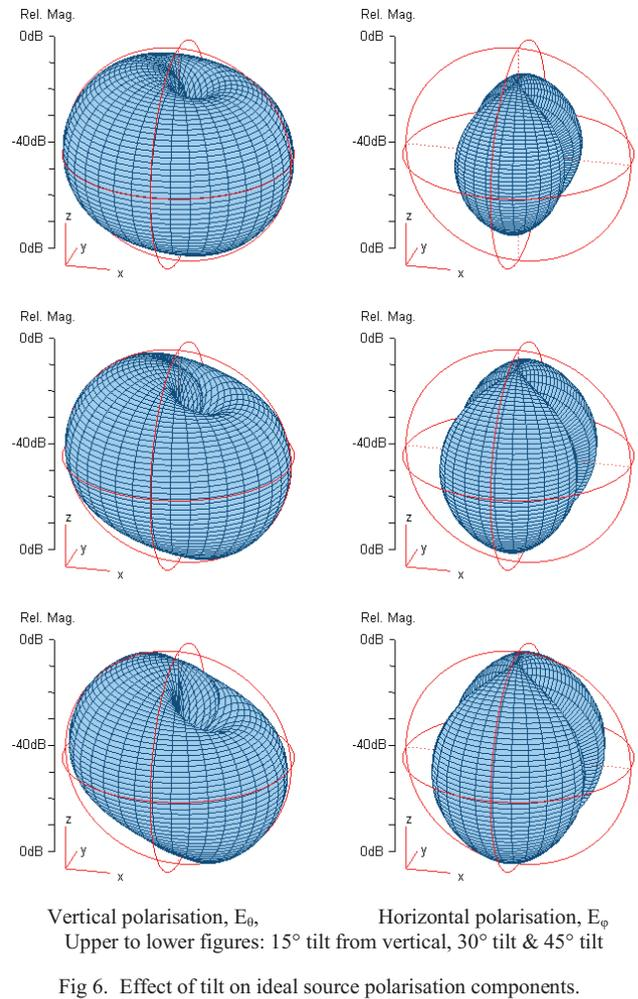
Fig. 6. Effect of tilt on ideal source polarisation components.
