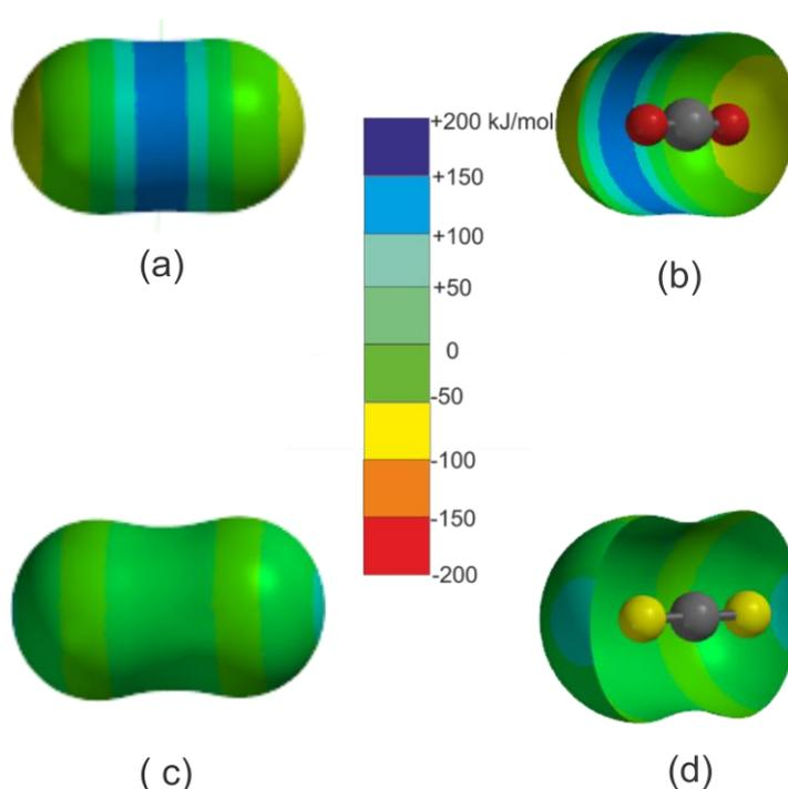
Figure 1. Molecular electrostatic surface potentials (MESPs) on the 0.002 e/bohr<sup>3</sup> of carbon dioxide (a) and (b) and carbon disulphide (c) and (d) calculated at the MP2/6-311++G\*\* level using SPARTAN. In (b) and (d), each surface has been rotated by several degrees about the C<sub>2</sub> axis and the front half removed.
