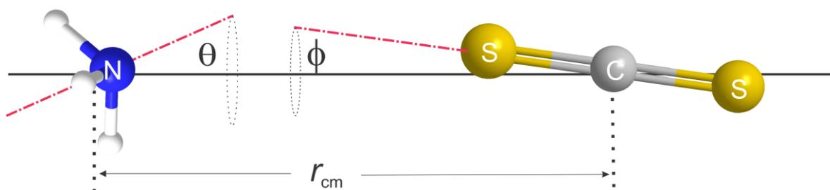
Figure 3. Definition of  $r_{\text{cm}}$  and the oscillation angles  $\theta$  and  $\phi$  used in interpretation of the observed principal moments of inertia  $I_b^0$  of 10 symmetric-top isotopologues of  $\text{H}_3\text{N}\cdots\text{S}=\text{C}=\text{S}$  to give  $r_{\text{cm}}$  and  $r(\text{N}\cdots\text{S})$ .
