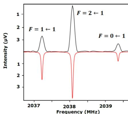
Figure 2. The  $J+1 \leftarrow J = 1 \leftarrow 0$  transition of the parent isotopologue of  $\text{H}_3\text{N}\cdots\text{S}=\text{C}=\text{S}$  showing the three  ${}^{14}\text{N}$  nuclear quadrupole hyperfine components. This was recorded by collecting  $1.15 \times 10^6$  free induction decays. The red spectrum is that simulated with PGOPHER by using the spectroscopic constants given in Table 1.
