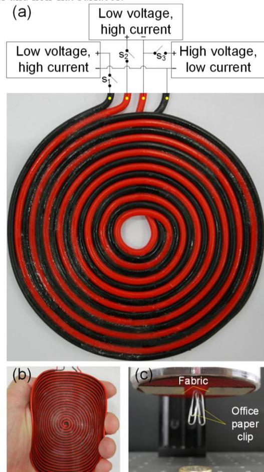
Fig. 1. Electro/Magneto-adhesive (E/MA) grippers. (a) The fundamental design of a monolithic and multi-modal E/MA gripper, with electric connections. (b) A flexible E/MA sheet gripper bent by hand. (c) Grasping magnetically susceptible (metal paper clips, total 0.80 g) and insusceptible (fabrics pieces, total 0.62 g) objects simultaneously using the E/MA gripper at 4.8 kV (high-voltage-low-current input) and 8 A (low-voltage-high-current input).
