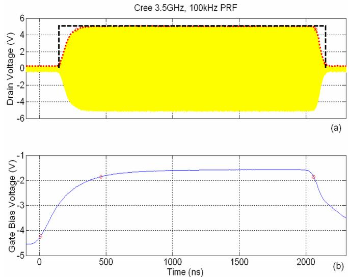
Fig 7 (a) Drain output at 9 dBm input power and 100 kHz PRF, Envelope (dotted), Ideal Envelope (dashed) – (b) Gate Bias
