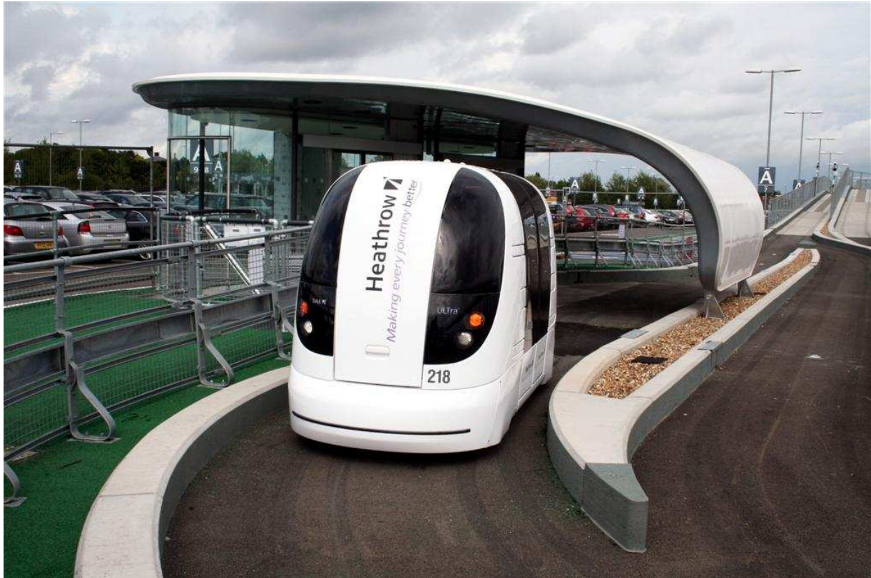
FIGURE 1 PRT vehicle and at-grade station at London Heathrow Airport. PRT vehicles, stations and infrastructure are smaller than typical Automated People Mover and urban rail systems. Vehicle length, width and height are 3.7m, 1.4m and 1.8m (12ft, 4.6ft and 5.9ft), respectively. Photo courtesy of Advanced Transport Systems Ltd.
