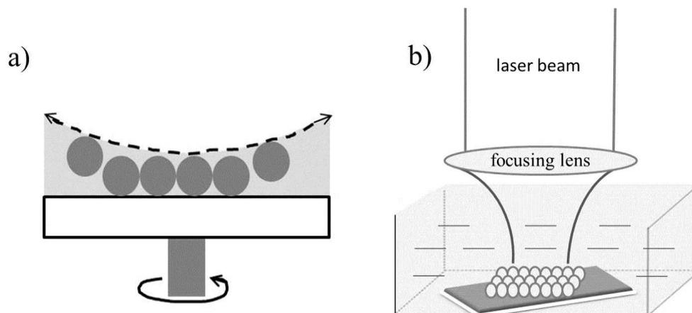
**Figure 1.** Schematic representation of the two steps involved in laser-initiated, liquid-assisted colloidal lithography: a) deposition of a close packed array of colloidal particles on a Si substrate and b) liquid-assisted, laser irradiation of a selected area of the Si surface beneath the colloidal particle array.
