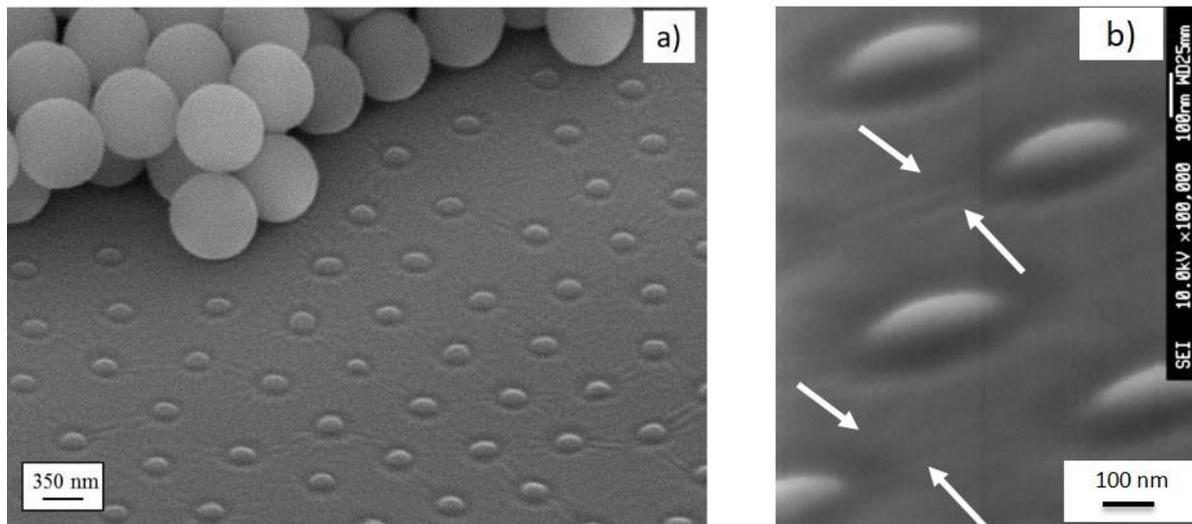
**Figure 6.** a) Overview and b) detail  $60^\circ$  tilt view SEM images showing the surface pattern achieved on Si by single shot LILAC lithography using a double layer of  $R = 350$  nm colloidal particles in  $\text{CH}_3\text{OH}$ , together with remaining particles at the periphery of the processed zone. Apparent hairline cracks are highlighted by arrows in b).
