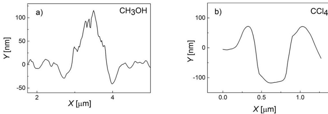
**Figure 5.** Line scan AFM traces of features formed by LILAC lithography of a Si substrate using an array of  $R = 1.5 \mu\text{m}$  colloidal particles: (a) a bump formed in  $\text{CH}_3\text{OH}$  and (b) a lipped hole formed in  $\text{CCl}_4$ .
