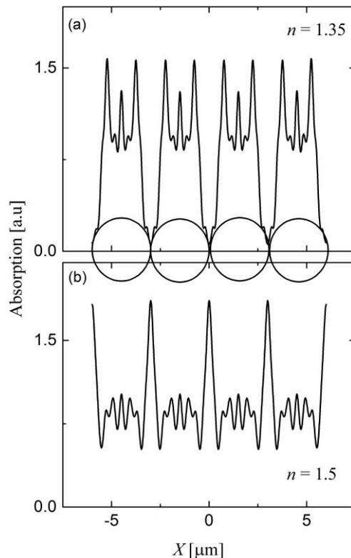
**Figure 3.** Cross-sectional view of the predicted absorption at the surface of a Si substrate located beneath a line (along  $X$ ) of four silica colloidal particles immersed in a liquid with (a)  $n_{liquid} < n_{colloid}$  and (b)  $n_{liquid} > n_{colloid}$ .
